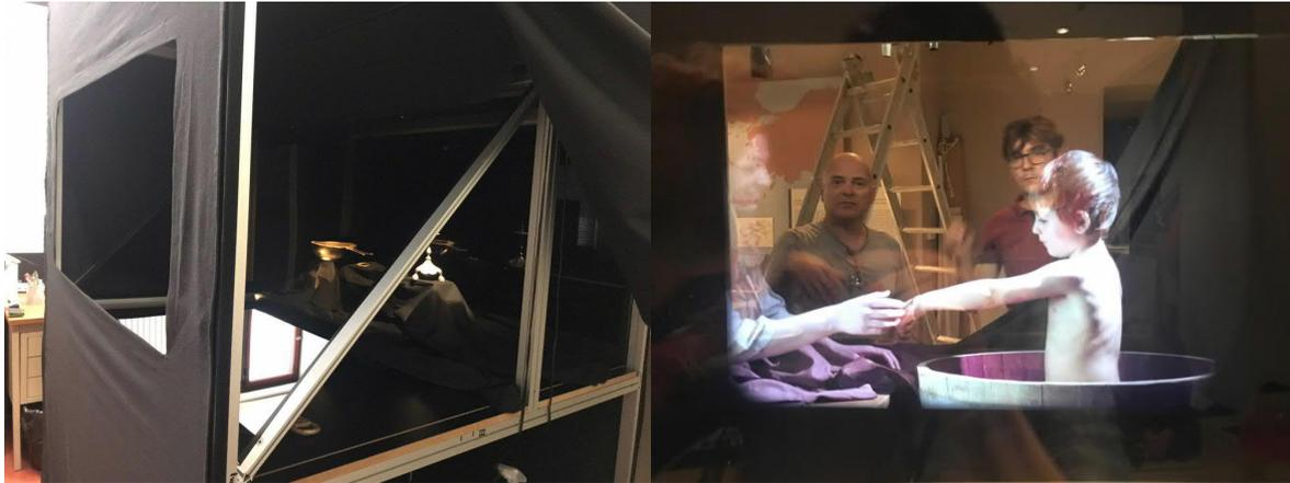
Fig. 3. a) Lateral picture of the holographic showcase with 45° glass, back objects and frontal glass clearly visible; b) effect produced by the transparent glass at the back of the structure
