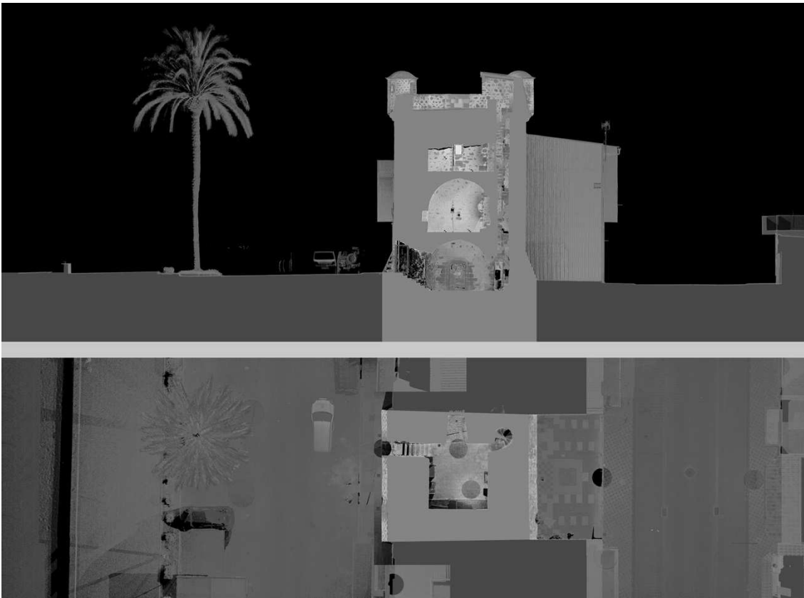
Fig 5 – Plan of the tower produced by Leica Cyclone
