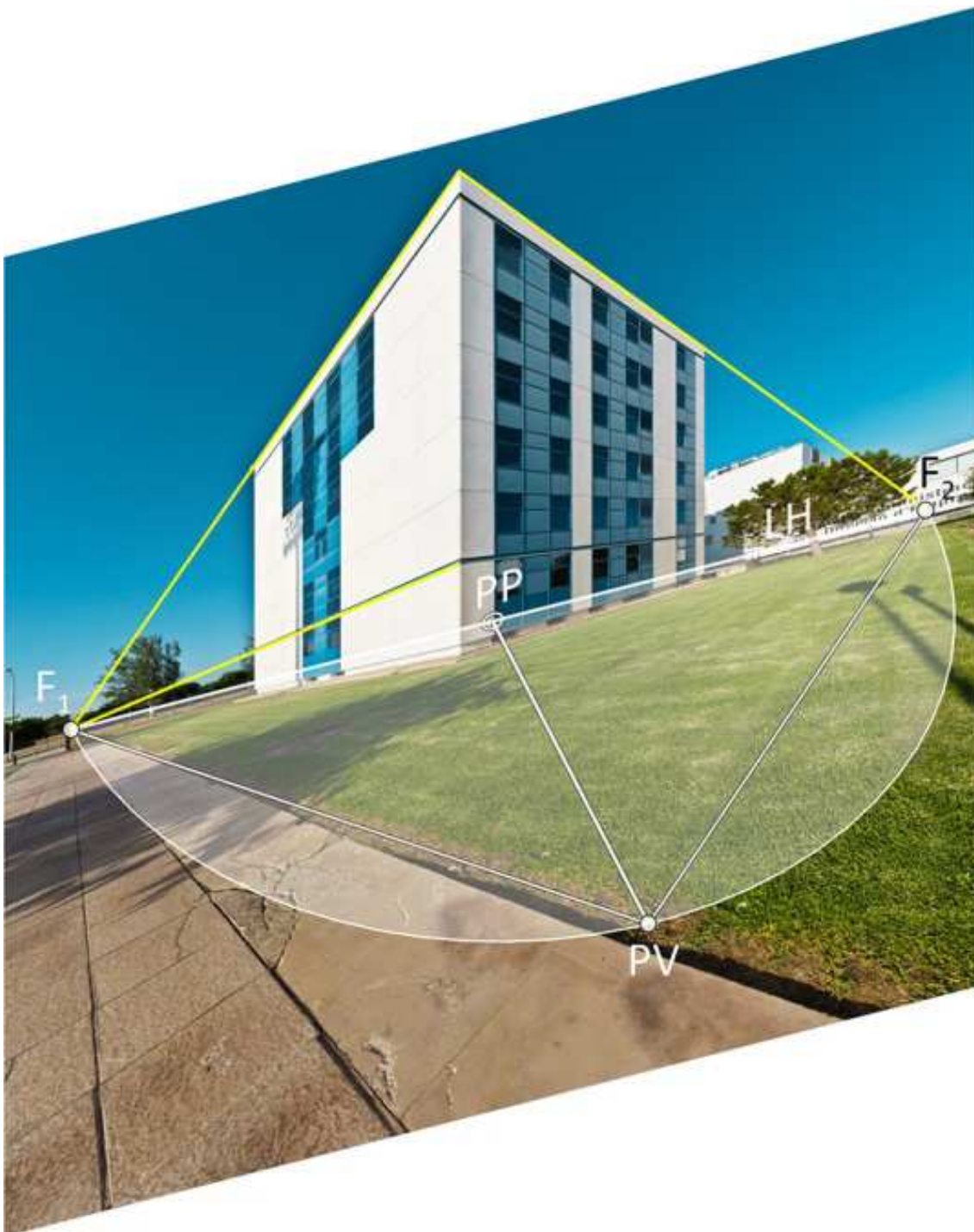
Fig. 3 – Perspective projection of a cube on a vertical surface (Pedro M. Cabezos-Bernal)
