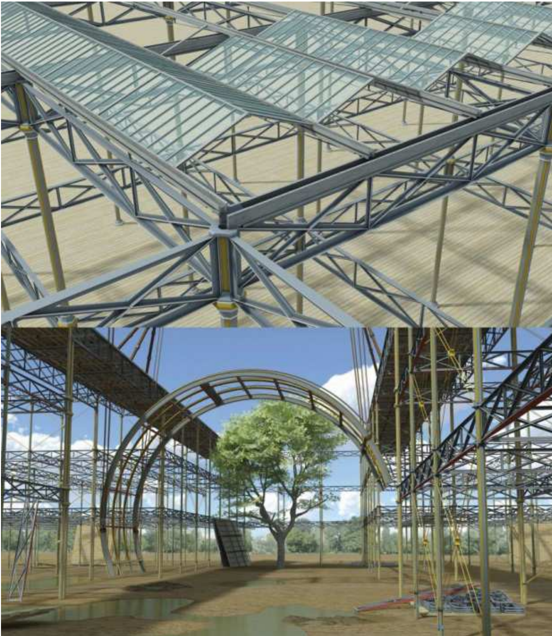
Fig. 3 – Construction elements of the Crystal Palace London, (Copyright TU Darmstadt, FG IKA, 2011)
