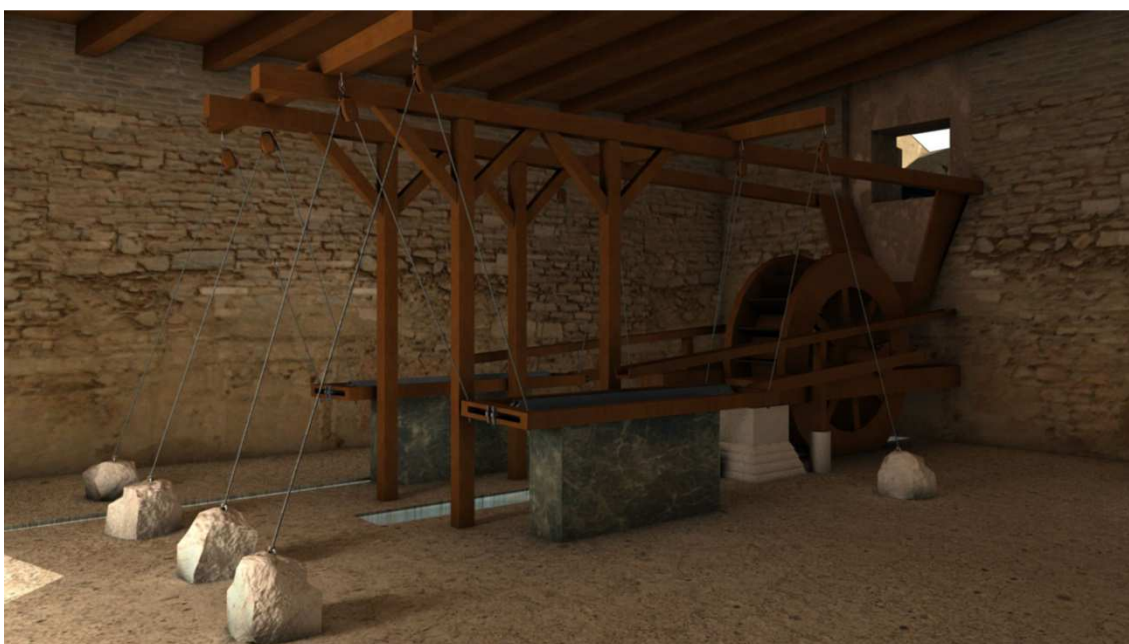
Fig. 2 – Digital reconstruction of the masonry saw in Ephesus (Copyright TU Darmstadt, FG IKA, 2012)
