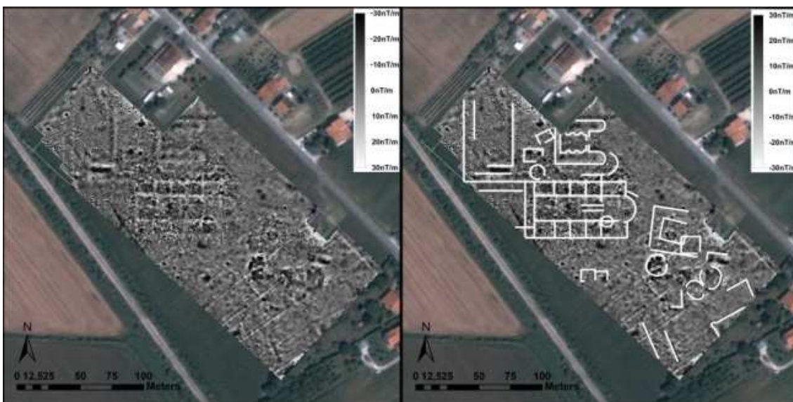
Fig. 10 – Area of the basilica Petriana. Magnetic map obtained with the Caesium magnetometer in the vertical gradient configuration, in collaboration with Helmut Becker (Becker Archaeological Prospection, Beuerberg, Germany), and interpretation of the main magnetic anomalies.
