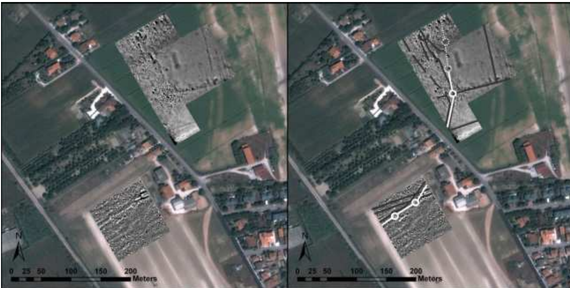
Fig. 11 – Area of the urban walls. Magnetic maps obtained with the Optically pumped Potassium Gradiometer and interpretation of the main magnetic anomalies.
