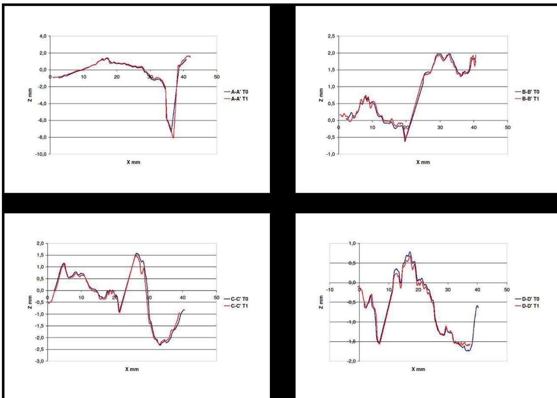
Fig. 8 – Overlapped sections of the crack measured in September 2011 and September 2012 with ZScan Micro technology (parish church of Saint Gavino Adimari).
