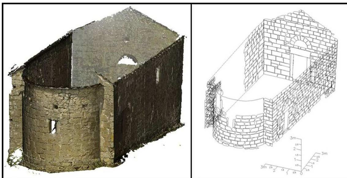
Fig. 5 – Example of three-dimensional model and of digitization in a 3D wireframe of the external façades of the church of Santa Maria a Fabbrica a Vicchio.
