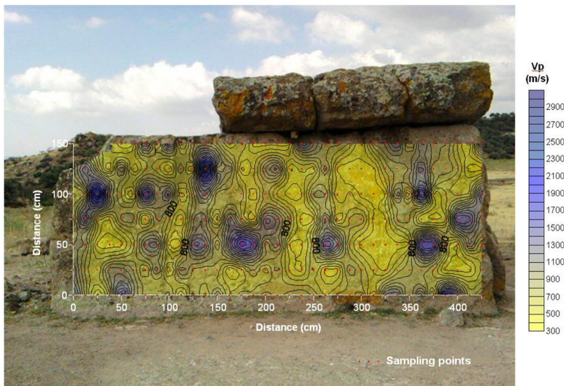
Fig. 7 – South ortostate of dolmen – longitudinal pulse velocity ( V_p ) map.
