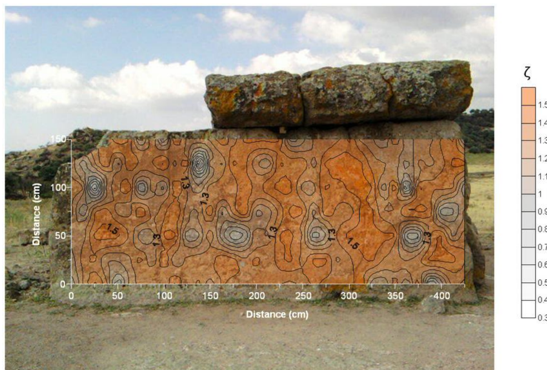
Fig. 8 – South ortostate of dolmen – map of fracture coefficient ( \zeta ).
