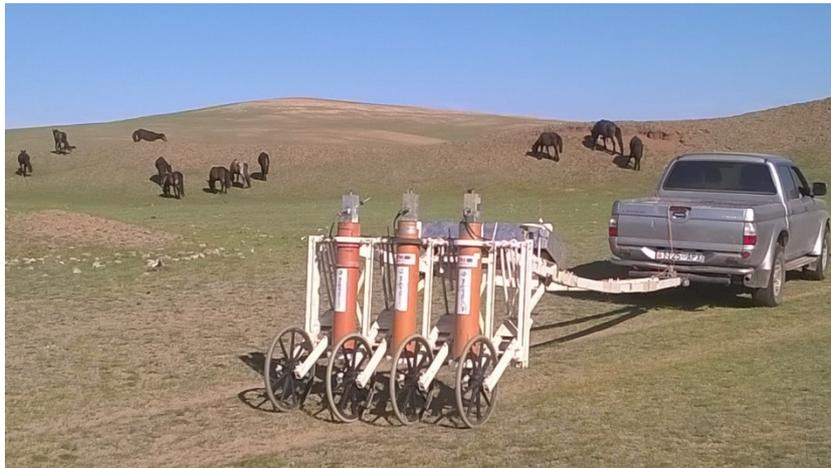
Fig. 1. The SQUID measuring system in operation nearby the main walled enclosure of Khar Khul Khaany Balgas, Mongolia. The three orange cryostates contain 18 magnetic field sensors within a scanning width of 1.5 meter (© Sven Linzen, Leibniz IPHT).
