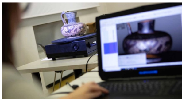
Fig 1: a structured-light 3D scanning was used to issue a geometric model of micrometric resolution in all its parts. The object was measured with 10 \mu\text{m} accuracy using an automatic turntable.
