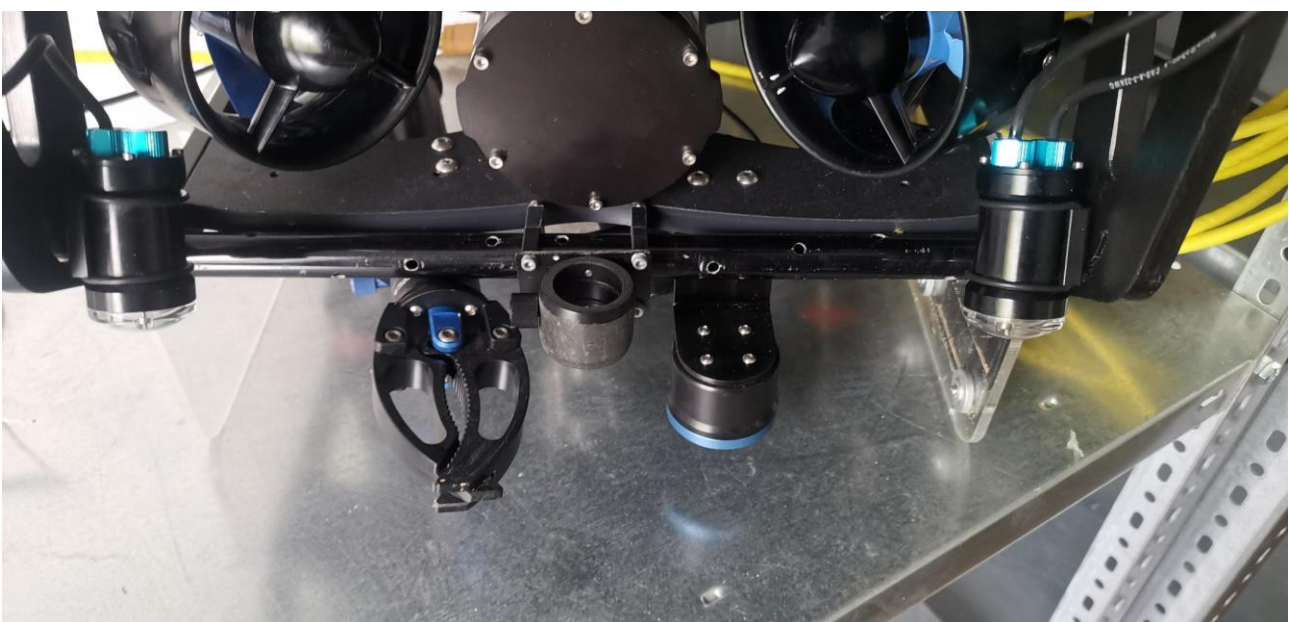
Fig. 3. On the left is the gripper arm with which sampling is currently possible. On the right is the sonar on the submarine, with which the distance to the bottom can be determined at any time.
