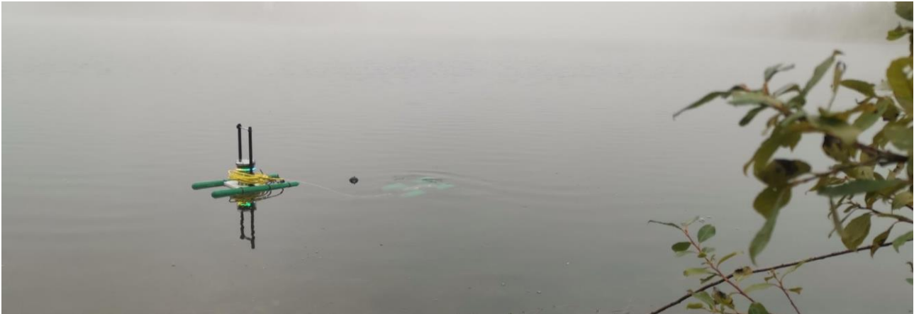
Fig. 1. current system with the bouy above water connected via a yellow cable with the submarine underwater
