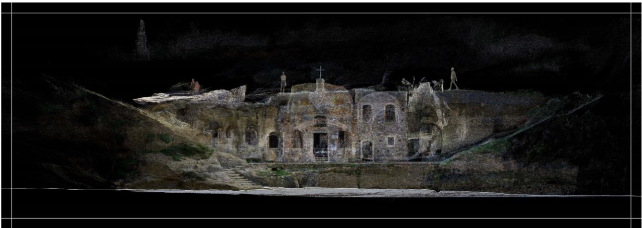
Fig. 1. Main elevation. Point cloud post-processing (elaboration of the authors).
