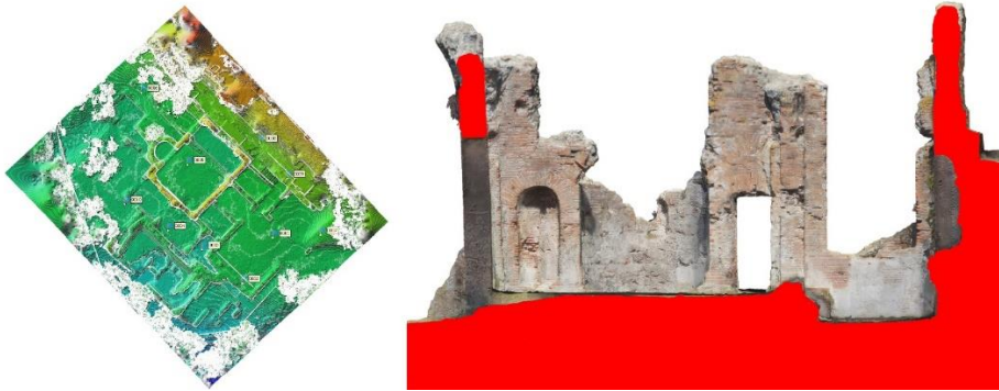
Fig.2 In this picture the DEM with contour lines and cross-section of the thermal complex elaborated from photogrammetric survey (Agisoft Metashape ®) is displayed.
