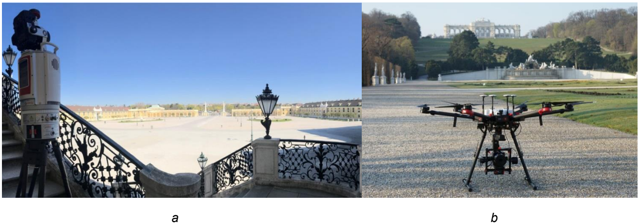
Fig. 1. a) TLS RIEGL VZ-400i; b) DJI Matrice 600 pro with Phase One iXM-100 camera
