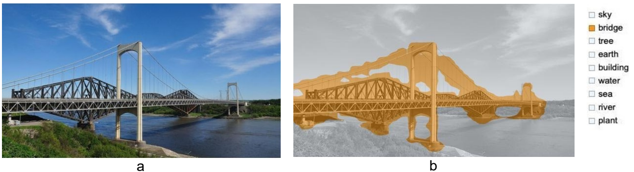
Fig. 2. Machine vision identification of bridge and other features a) original image; b) identified features.
