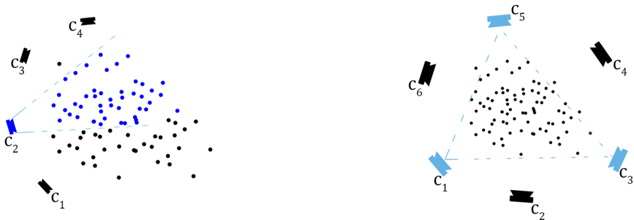
Fig. 3. Four camera positions can be seen on the left, with blue being the well-referenced ones. C_2 is a well-referenced camera position. Therefore, all points recorded by this camera are considered good. In the right picture, three furthest camera positions are highlighted to be selected for referencing the model.
