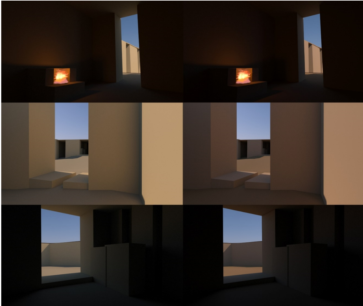
Fig. 1. Mudbrick/plastered walls and dirt ground, as seen from indoor and outdoor angles, modeled with brown color from an on-site reference photo using the Photoshop dropper tool (left) vs. accurate BRDFs under sunlight dome conditions (right).
