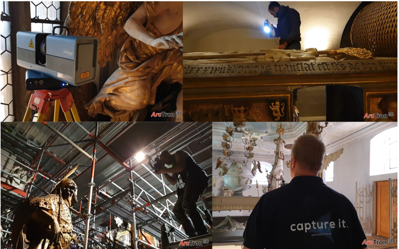
Fig. 2. 3D scanning with different technologies: laser scanning (Surphaser), handheld structured light scans (Artec EVA), photogrammetry, indoor drone-flying (ArcTron 3D GmbH).
