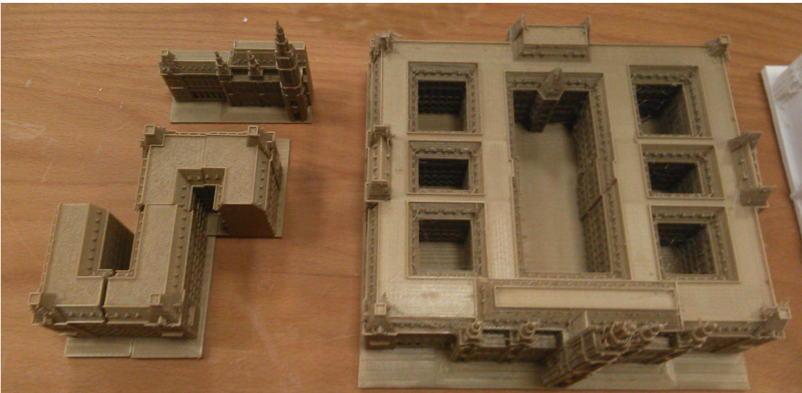
Fig. 7 – Printed results, on the left: Makerbot 2nd, on the right: Makerbot z18.
