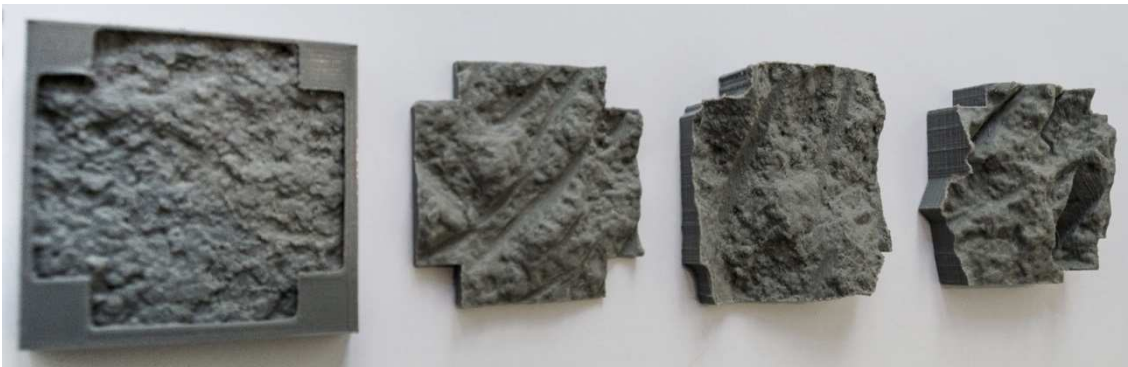
Fig. 9 – 3D printed of the stone manufacturing samples (Copyright: Andrea Pasquali - Angela Mancuso)
