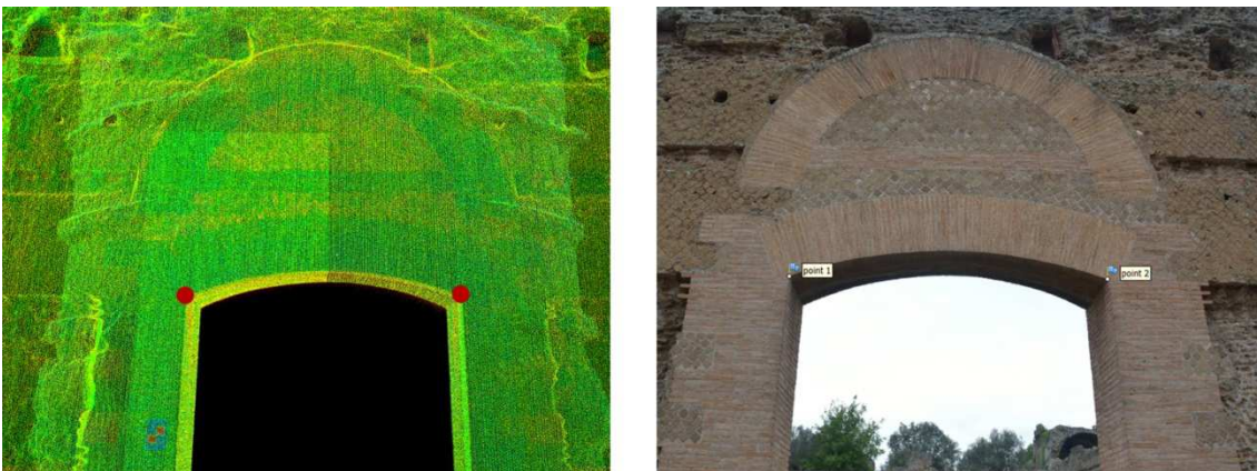
Fig. 3 – Reference point between point cloud and photogrammetry model
