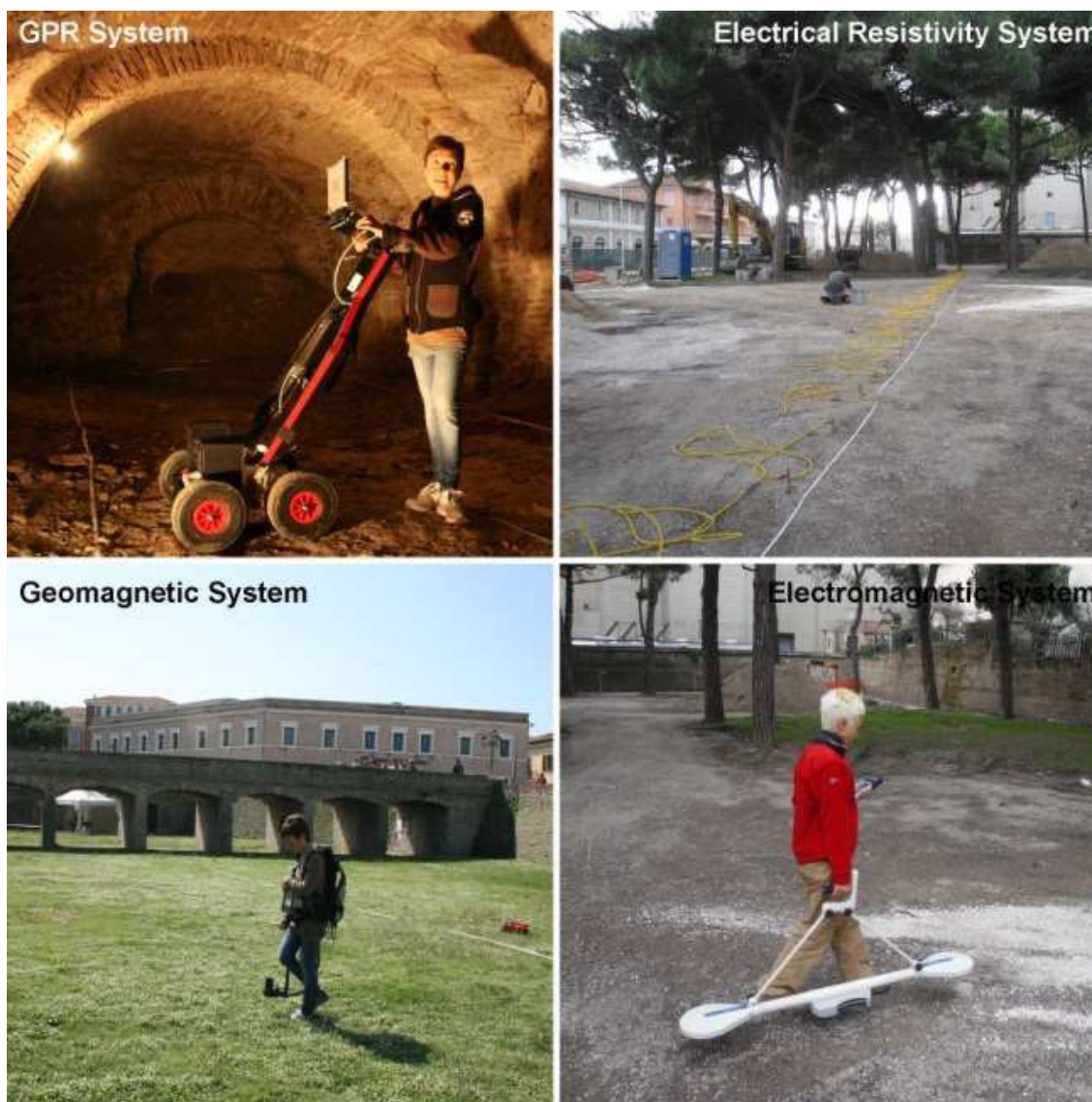
Fig. 5 – Integration of different geophysical systems applied to the urban area.
