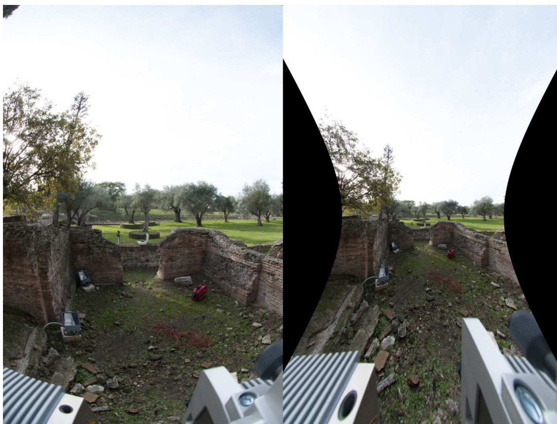
Fig. 17 – a fisheye picture before and after the lens correction
