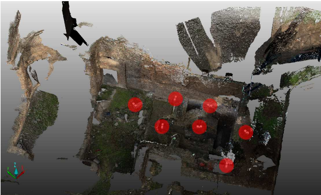
Fig. 11 – The full pointcloud of the boiler room with in red the seven scanstations
