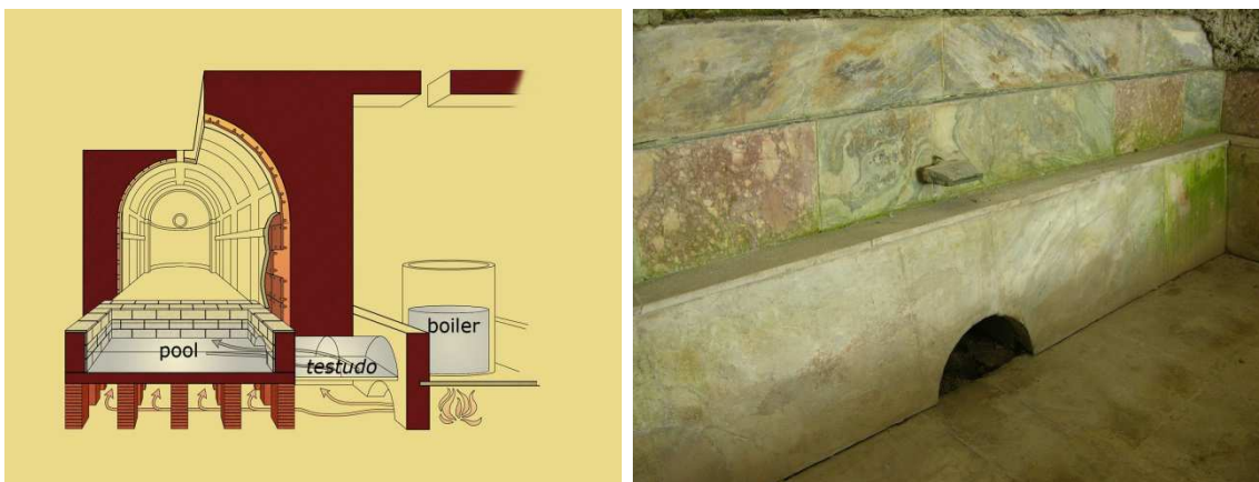
Fig. 7-8 – The testudo in a reconstruction and in the Suburban Baths in Herculaneum
