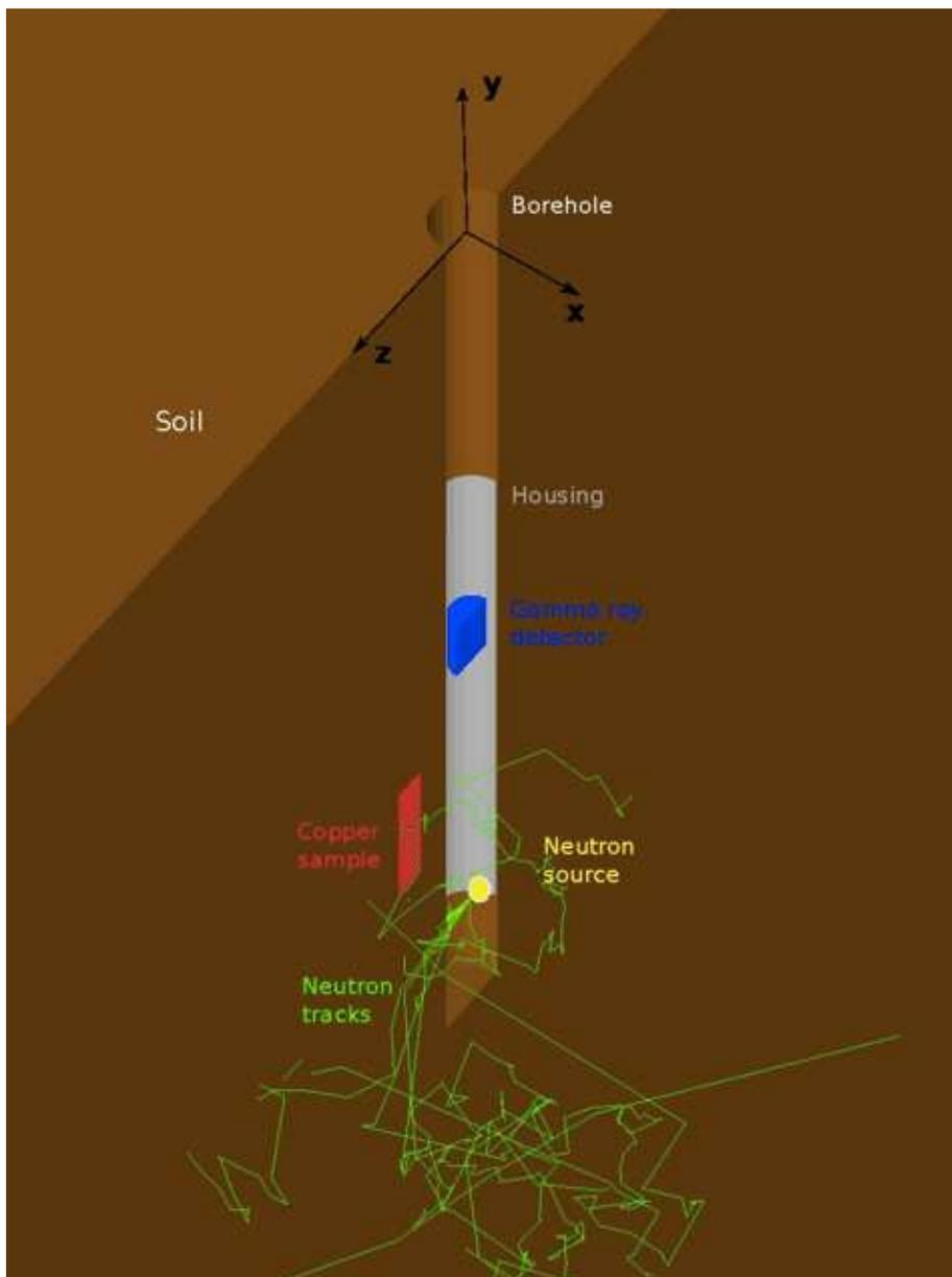
Fig. 1 – Geant4 model of the neutron logging system. Gamma detector (blue), neutron source (yellow), and logging system housing (gray) inside the borehole, and copper sample (red) buried in the soil (brown) are illustrated. The green lines indicate the neutrons interacting with the soil and the sample. The visualization was generated with the Geant4 DAWN and DAWNCUT visualization tools.
