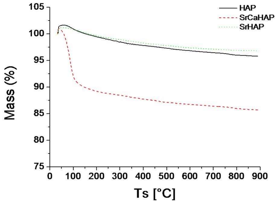
Fig. 7 – Thermogravimetric analysis results for HAP/SrCaHAP/SrHAP
