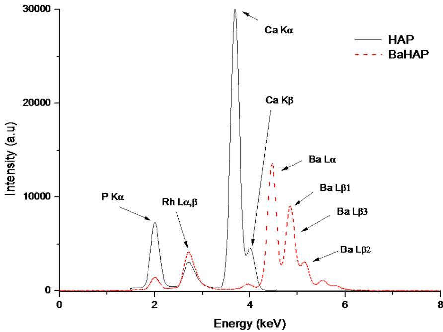
Fig. 2 – EDXRF results for HAP/BaHAP
