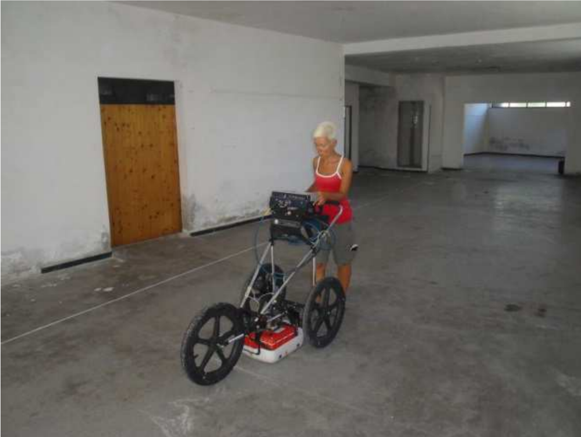
Fig. 2 – Data acquisition with the ground penetrating radar GSSI SIR 3000.
