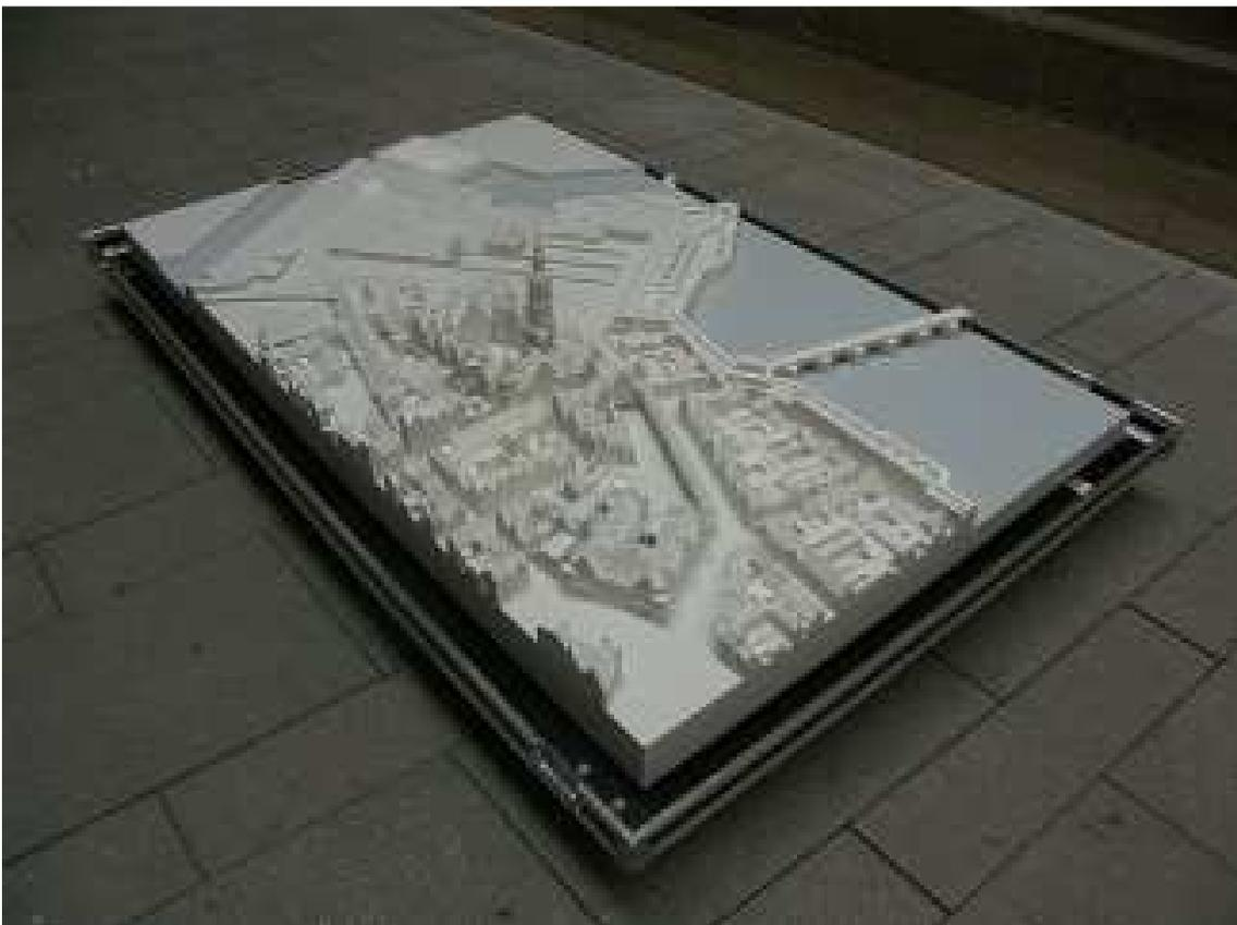
Fig. 11 – Rapid Prototyping Model of Dresden 1678 (Copyright: FG IKA, TU Darmstadt)
