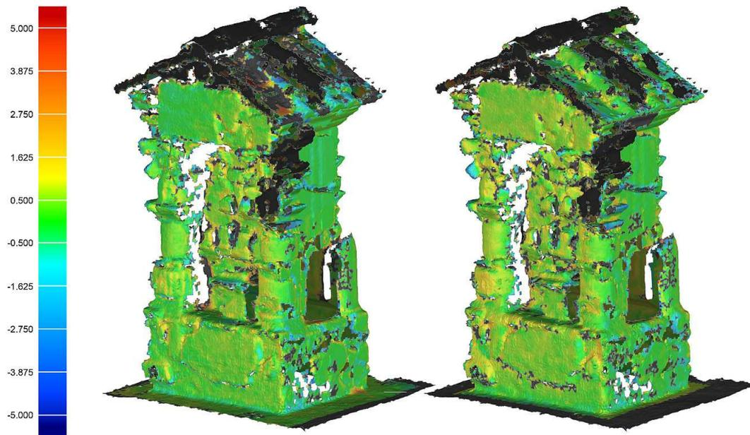
Fig. 5 – Results of the accuracy test on 123D Catch model (left) and Photoscan model (right)
